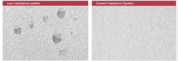
The hail resistance of any component is rated with classification system called Hail Impact Resistance (HIR). The rating defines the energy at which the facade still shows no damage. Ceresit Impactum System, even with smaller diameter of the ball, outranks HW 5 class – the highest resistance rating for hail.
